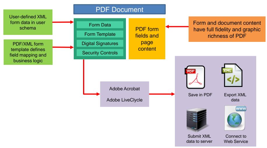
An XDP file is an XML file that packages a PDF file in XML, along with XML form and template data. Since an XDP file is an XML file, standard XML tools, system interfaces, and Web services can work with it, making the XML data directly accessible.
