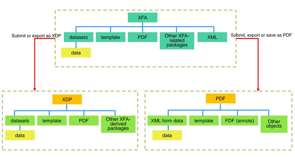
When an XFA processing application is requested to submit or export XFA components, it packages those components as an XDP document (below left) or as a single PDF document (below right). XDP and PDF can represent the same XFA form component; however, they differ in their root nodes and in the compliance with XML. That is, XDP is XML-compliant, while PDF is not.
